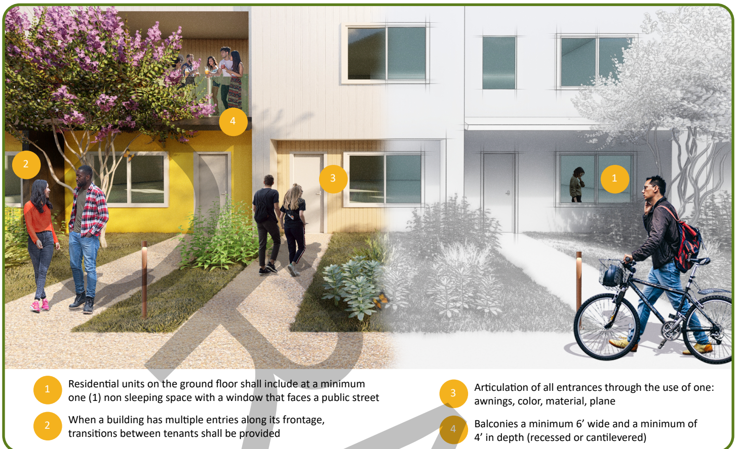
Figure 2-26: Building Articulation and Massing
